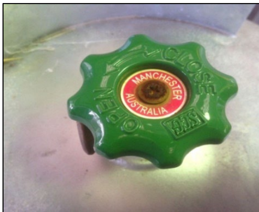
Figure 40. Exchangeable gas cylinder showing green tap with 'OPEN' and 'CLOSE' markings
