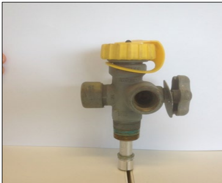
Figure 39. In-situ gas cylinder showing removable yellow cap
