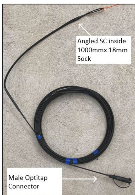
Figure 56. CCC with HFOC (Hardened Fibre Optical Connector)
