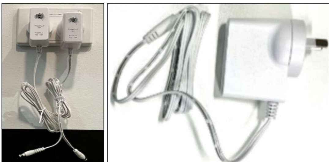
Figure 11. Nokia and Sercomm 1 and 4-port NTD 12V DC PSU
