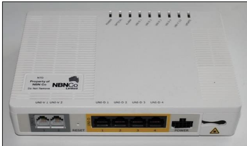
Figure 10. nbn® GPON Ethernet legacy NTD
